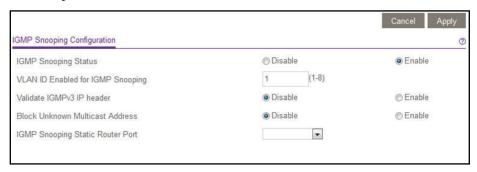
6. Make sure that the IGMP Snooping Status **Enable** radio button is selected.
