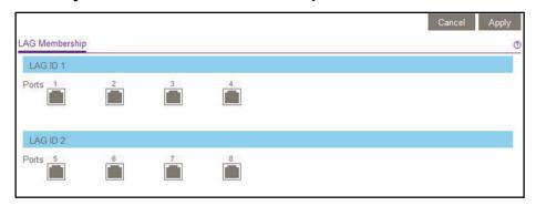
**Note:** Model GSS108EPP provide 8 ports and can support up to 4 ports per LAG. Model GSS116E provides 16 ports and can support up to 8 ports per LAG.
