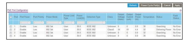
The delivered power is stated in the Output Power (W) column (4.4W for Port 2 in the previous figure).
